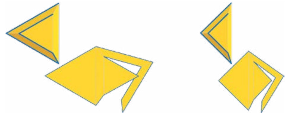
Figure 3. The left side shows a truncated tetrahedron (viewed from "above") together with an overlapping unfolding of it generated by a monotone edge tree. As we see on the right side, however, the same edge tree generates a simple unfolding once the polyhedron has been stretched.
